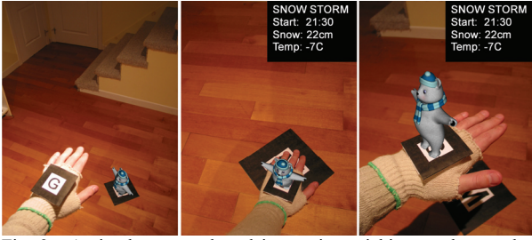
Fig. 2. A simple gesture-based interaction: picking-up the weather avatar on the floor to indicate interest for this software process.
